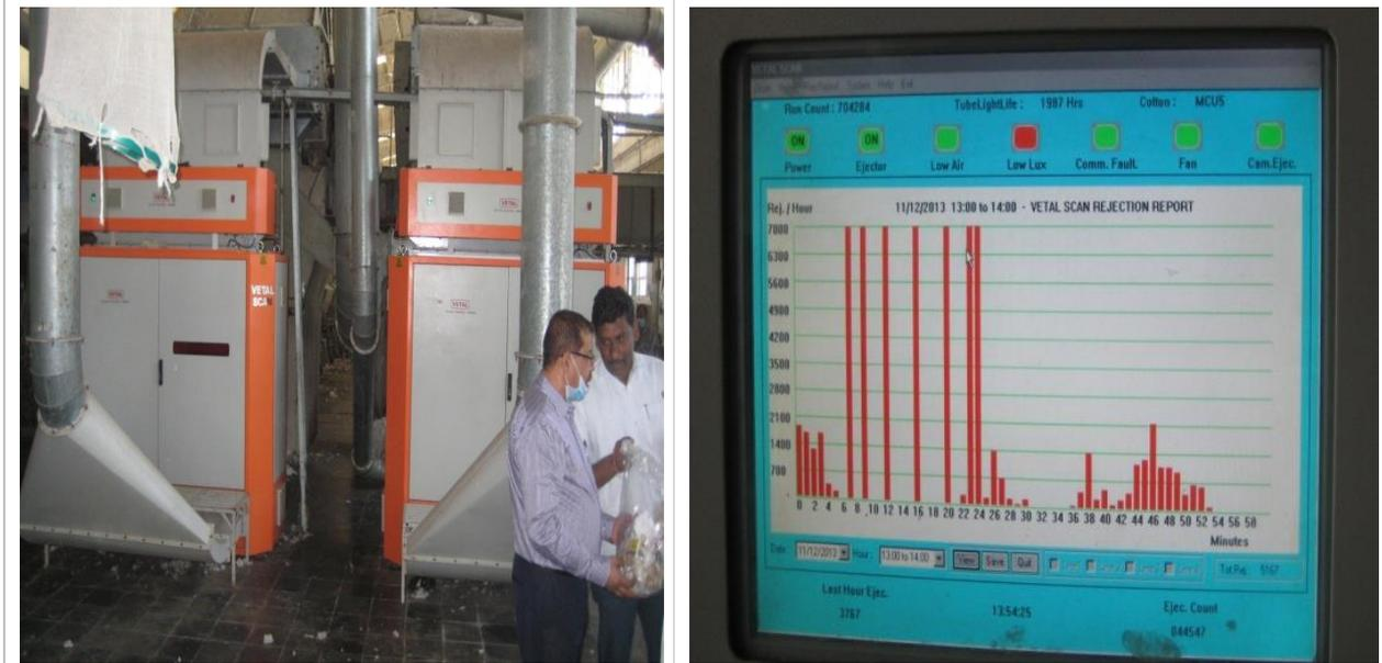
Contamination Cleaning Machines: the machine is suitable for both ginning and textile mills. The machine, when in operation, generates automatic contaminants rejection reports
