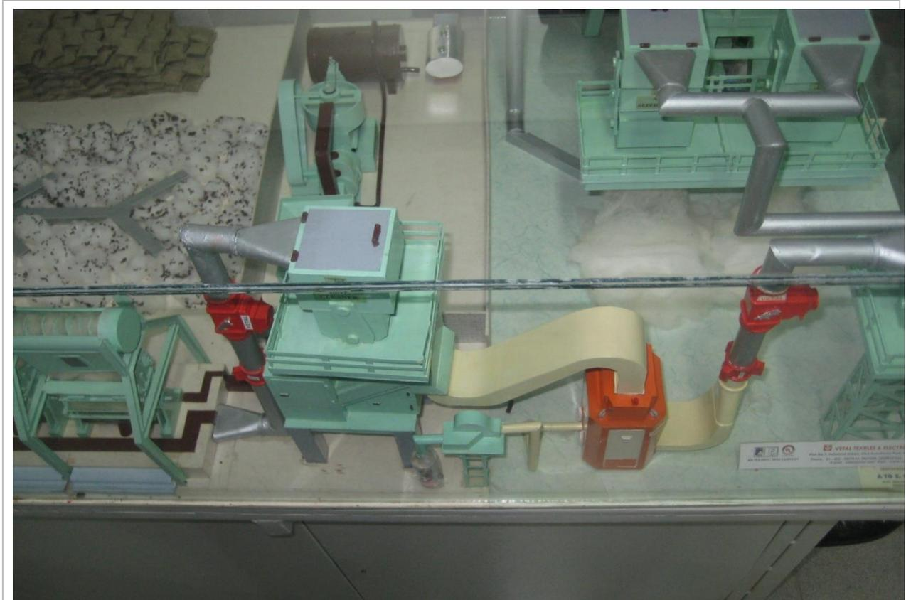
Ginners layout showing the position of the contamination cleaning machine
