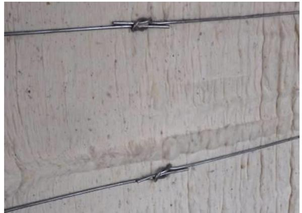
Steel wires should not be used for bailing. Cotton is sensitive to contamination by rust. Moreover, steel straps could cause fires in a spinning factory when opened by force
